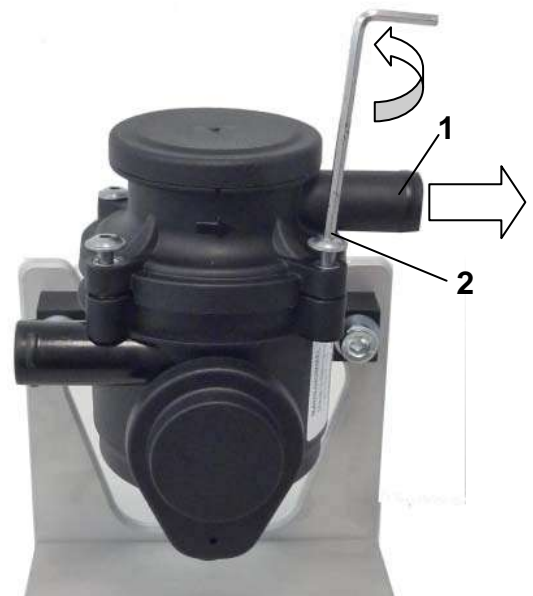
Fig. 10 Detaching lid of ProVent 100
