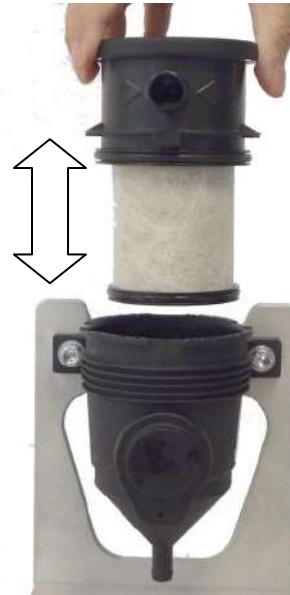
Fig. 13 Changing oil separator of ProVent 150
