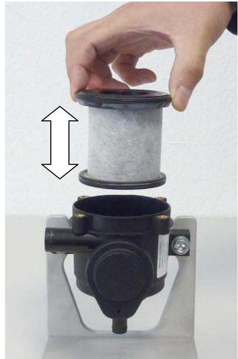
Fig. 11 Changing oil separator of ProVent 100
