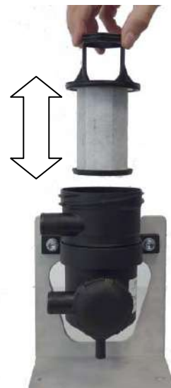
Fig. 15 Changing oil separator of ProVent 200
